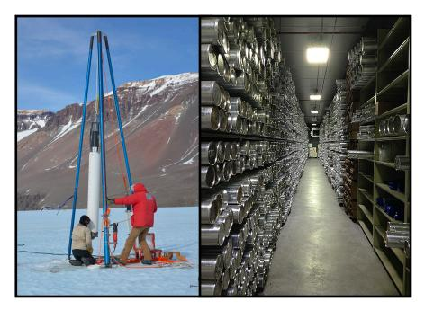
This facility has a giant freezer that stores ice cores at 36 degrees below zero. They collect samples from around the world for testing and one of those places is Greenland. They take a very long pipe and drill into the ice and pull it out and store it for testing.
